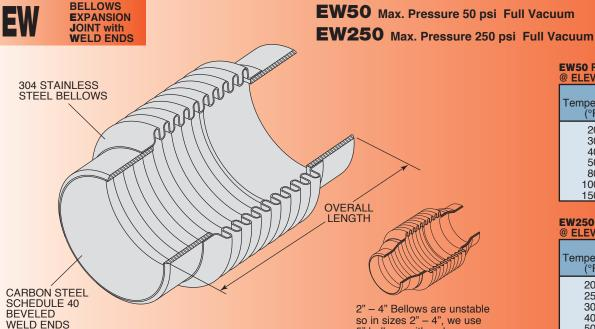
so in sizes  $2^{"} - 4^{"}$ , we use 5" bellows with reducers on each end to avoid buckling.
