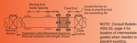
Guides and Anchors for Joint located between Remote Anchors
