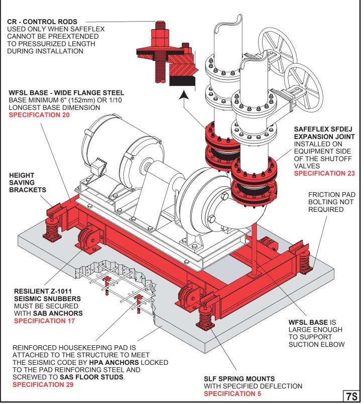
**END SUCTION PUMP** on **WFSL** Base with height saving brackets, **MT** Air Springs and **Z-1011** Seismic Restraints. Reinforced housekeeping pad secured by **HPA** Anchors. **SAFEFLEX** Expansion Joints are installed in pipelines to reduce blade frequency vibration and noise and to allow for seismic displacement.
