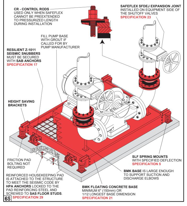
**END SUCTION PUMP** on **WFSL** Base with height saving brackets, high deflection **SLF** Mounts and **Z-1011** Seismic Restraints. Reinforced housekeeping pad secured by **HPA** Anchors. **SAFEFLEX** Expansion Joints are installed in pipelines to reduce blade frequency vibration and noise and to allow for seismic displacement.
